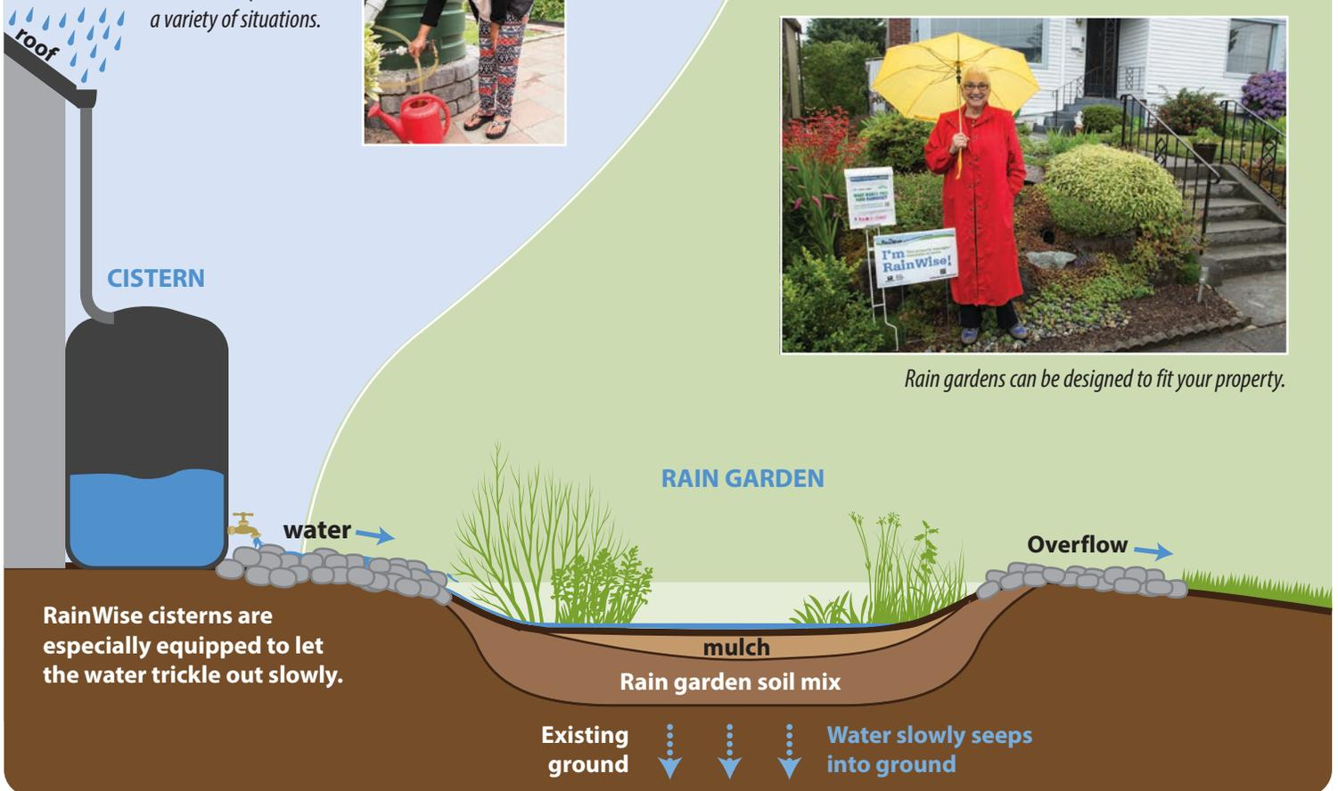
RainWise cisterns are especially equipped to let the water trickle out slowly.
