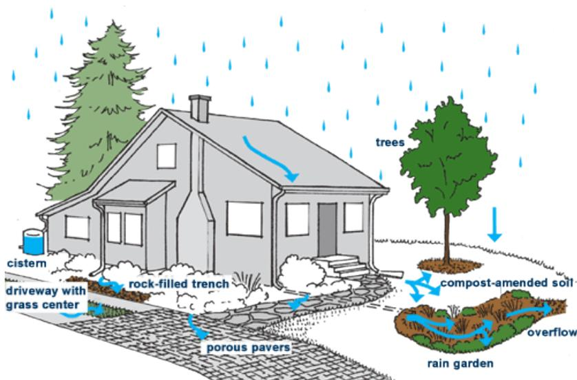
The **Stormwater Features Diagram** shows solutions people might use to help with stormwater problems. Some solutions involve plants and soil (trees, rain garden, compost-amended soil, driveway with grass center) and others do not (rock-filled trench, porous pavement, cistern). All are intended to slow down, spread out, and filter rain water so that it does not cause flooding.
