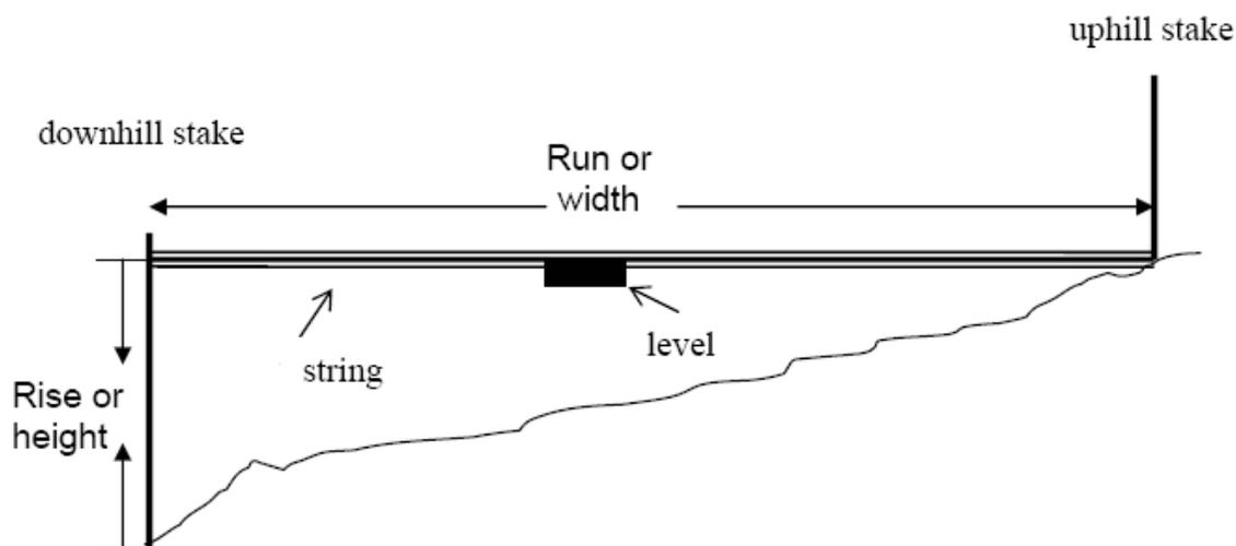
The percent slope is calculated by measuring the change in height (elevation) over a measured distance. The following formula determines slope:
