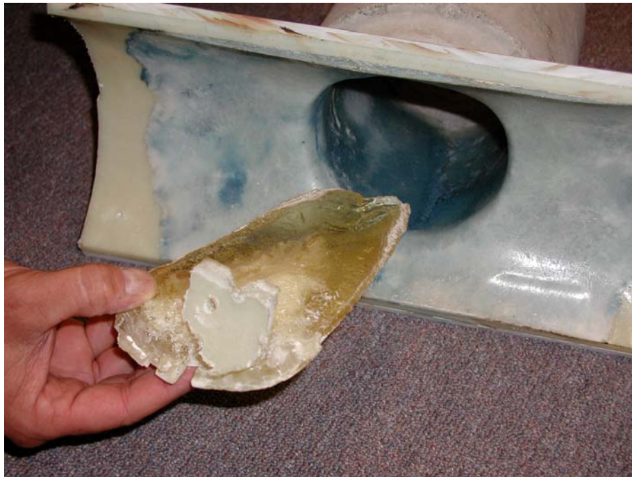
Epoxy resin slug that pooled in a lateral connection to a sewer main during the installation of the CIPP in the sewer main. The slug is held adjacent to a sample pipe section with a lateral connection to illustrate the location of the slug in the field. The slug was removed during the reinstatement of the lateral connection.
