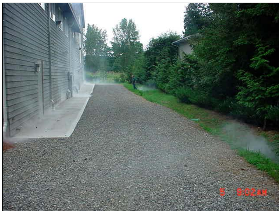
Smoke emanating from ground during smoke testing.
