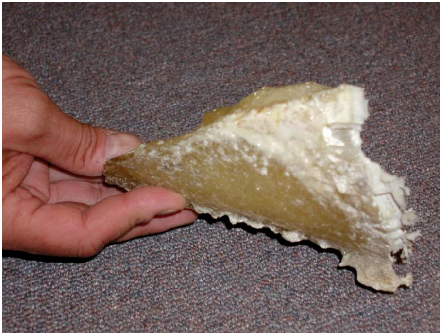
Epoxy resin slug removed from laterals.
