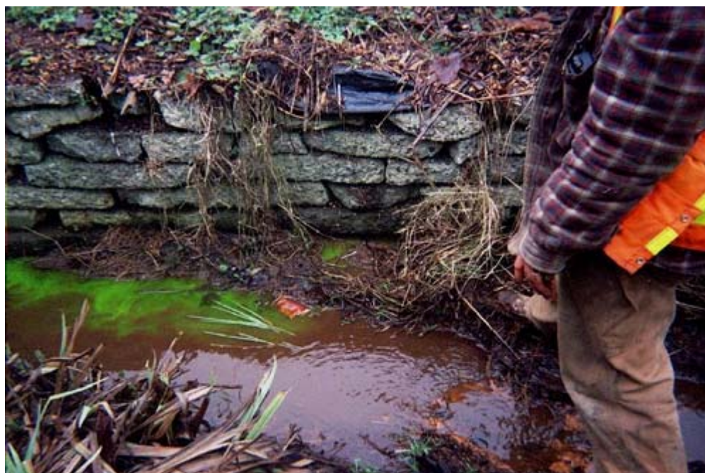
Dye testing confirming down spout connected to ditch rather than sanitary sewer.
