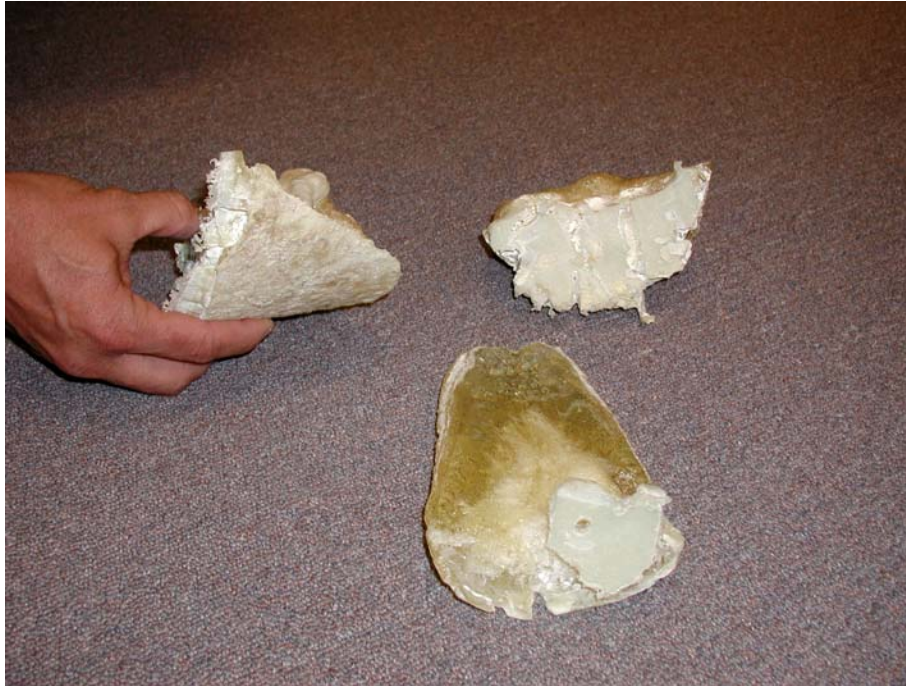
Epoxy resin slugs removed from laterals.
