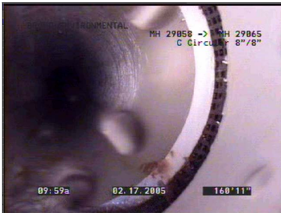
Figure 4 – Non-HDPE coupling used during pipe busting Used for the joint immediately outside a manhole in Kirkland.
