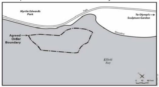
About 20,000 cubic yards of material contaminated with PCBs and mercury must be removed. The county contractor will use a mechanical dredge on a barge to excavate the area and load contaminated sediment onto a second barge. This second barge will transfer the sediment to trucks for transport by rail to a landfill. The excavated area will be backfilled with clean sand and gravel to match the seabed's existing grade and improve the site as shallow-water nearshore habitat.
