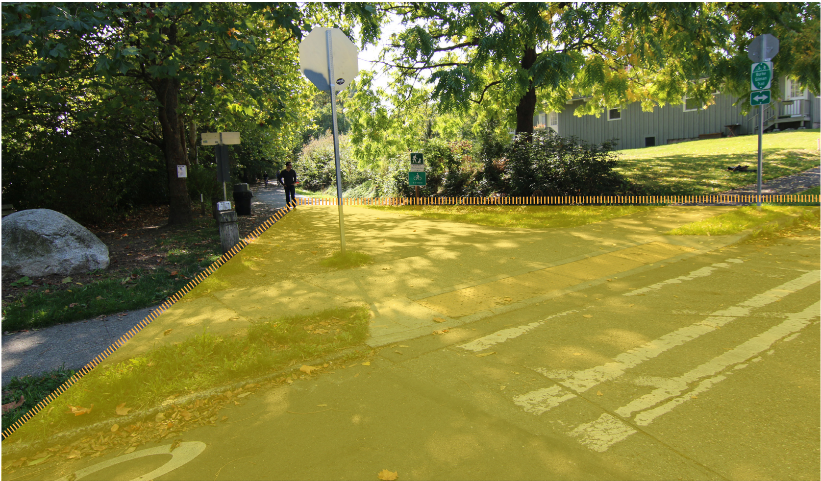
Pedestrian on trail must be able to see approaching vehicles in both directions at intersections.
