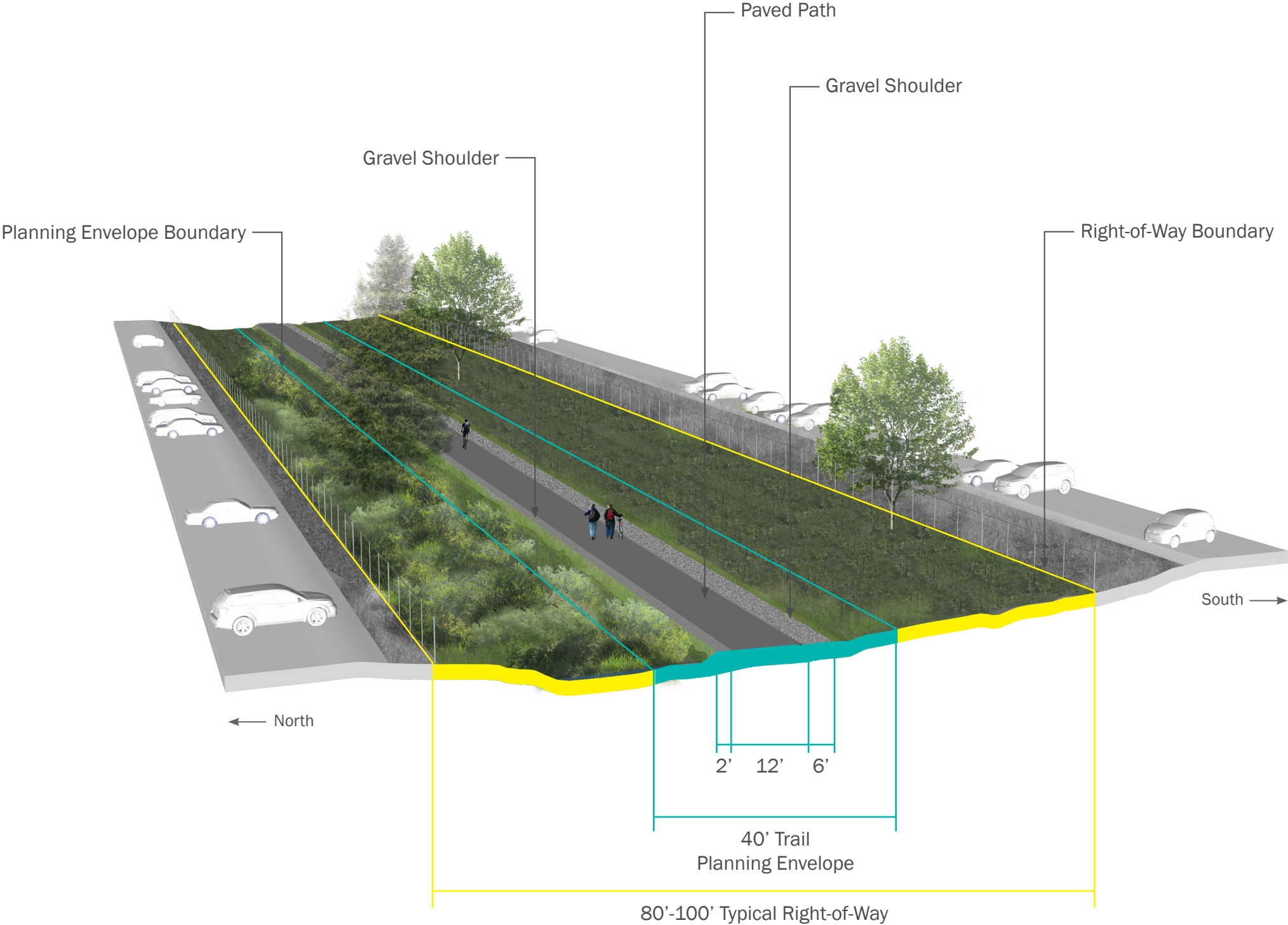
FIGURE 4-18. VALLEY SEGMENT – MAIN LINE SECTION 1, ON-RAILBED ALTERNATIVE
