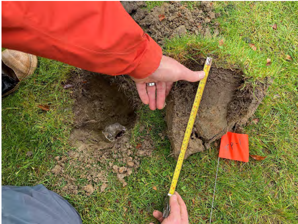
Photo 1—Soil profile at TP-1.
